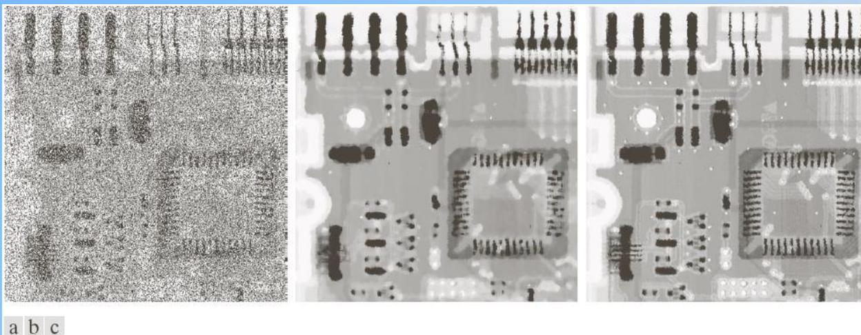
**FIGURE 5.14** (a) Image corrupted by salt-and-pepper noise with probabilities  $P_a = P_b = 0.25$ . (b) Result of filtering with a  $7 \times 7$  median filter. (c) Result of adaptive median filtering with  $S_{\max} = 7$ .
